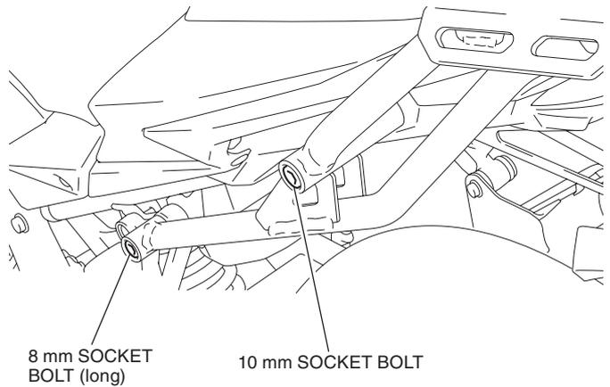
6. Securely tighten the 8 mm socket bolts as shown.
