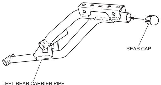
3. Loosely install the left rear carrier pipe as shown.
