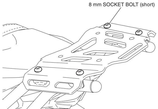
7. Install the socket bolt caps as shown.
