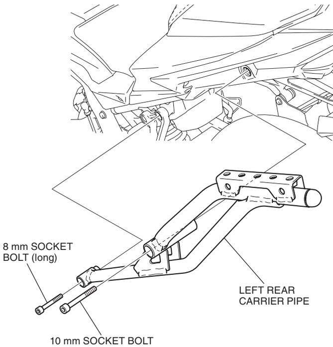
4. Loosely install the rear carrier plate as shown.
