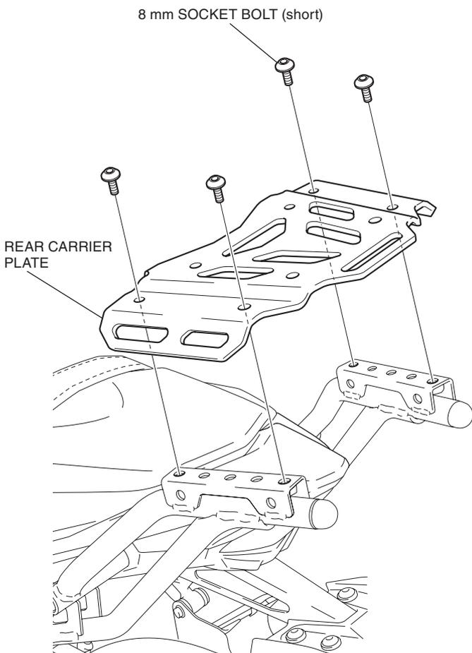
5. Securely tighten the 8 mm and 10 mm socket bolt as shown.
